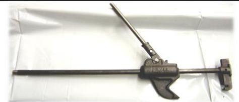
Barbed Wire / Tension Wire Puller TWG
